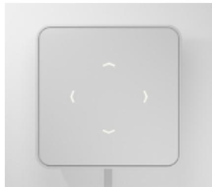
In this menu, the LED ring will light up purple and 4 arrows will be displayed. Use the top arrow when you want to install your device via WPS. Use the bottom arrow if you want to reset the Wi-Fi.
